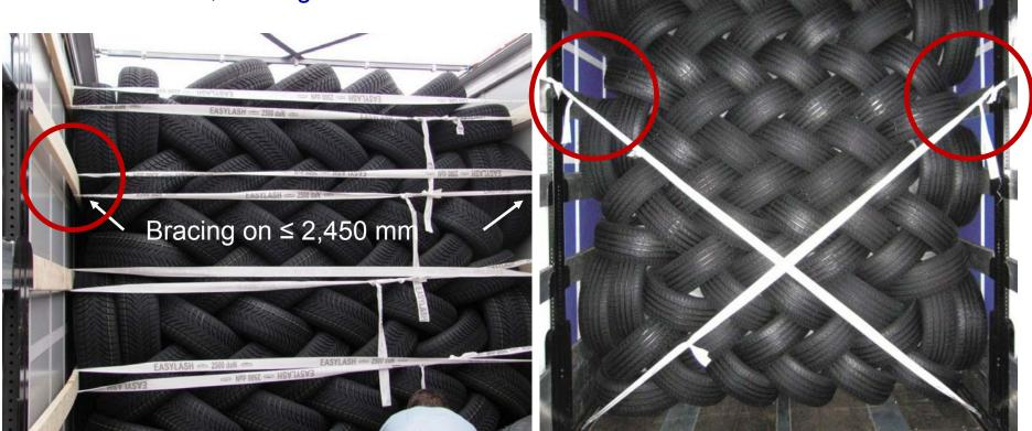
disposable lashings type EasyLash® (2,500 daN in loop strapping) ordouble PP-Cord (Hanfwolf Type MNM<br/>032/single, elongation at break 120 daN)50 mm lashing straps in line with<br/>DIN EN 12195-2, LC 2,500 daN
