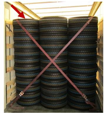
Diagonally crossed belts using 2 lashing straps which are hooked left and right in traveling direction into the lashing points of the vehicle. The straps are passed over the outermost tyre columns hooked into the lashing points of the vehicle and finally tensioned.
