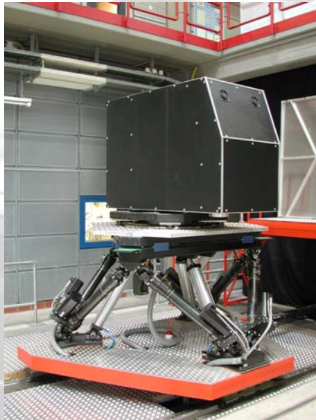
Dynamic Driving Simulator; 8 DoF
