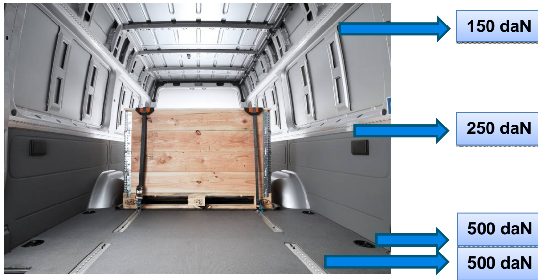
Serial equipment with lashing points in all commercial vans according to ISO 27956
